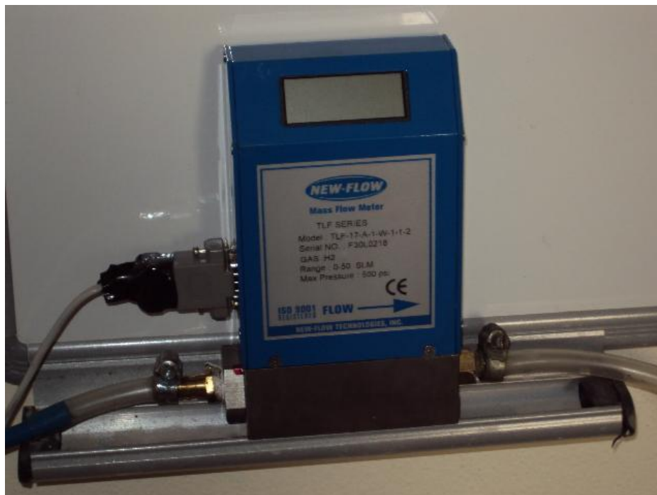
Figure 4.12. Electronic hydrogen flowmeter
