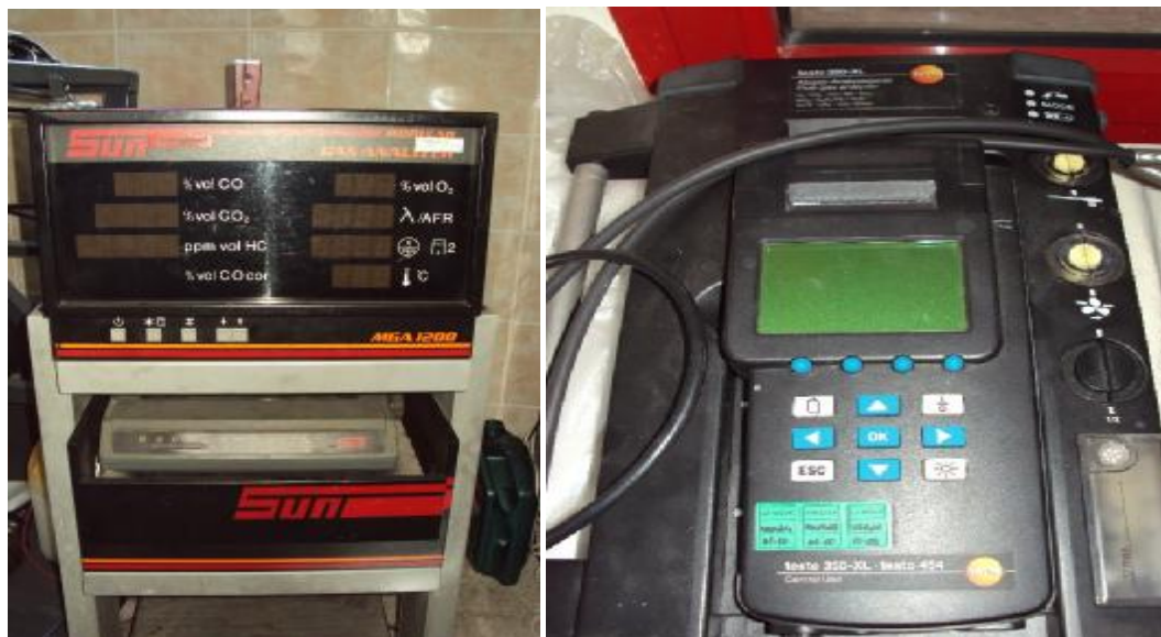
Figure 4.11. Gas analyzers of SI and CI engines
